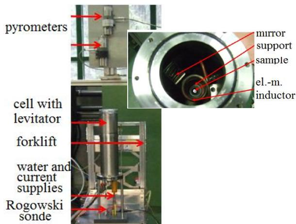
Fig.1 Setup for the measurement of the thermophysical properties on levitated samples
