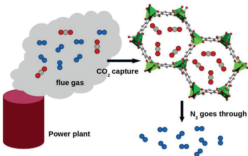
*Sketch of a postcombustion capture process that uses MOFs. The flue gas contains 15 % of CO<sub>2</sub> and 75 % of N<sub>2</sub>. Due to the low pressure of the flue gas (1 atm), the MOF should exhibit an extremely high affinity for CO<sub>2</sub> which can be modified with light treatment.*
