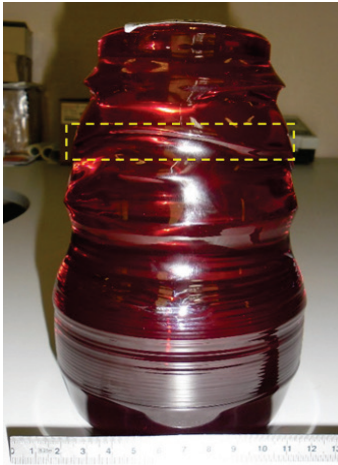
Fig. 1: 100m diameter sapphire single crystal doped with Ti for ultra-high power lasers. Courtesy RSA company.
