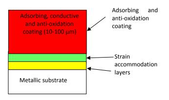
Selection of a conductive, adsorbing and oxidation-resistant material: AIN and SiC are the first candidates
