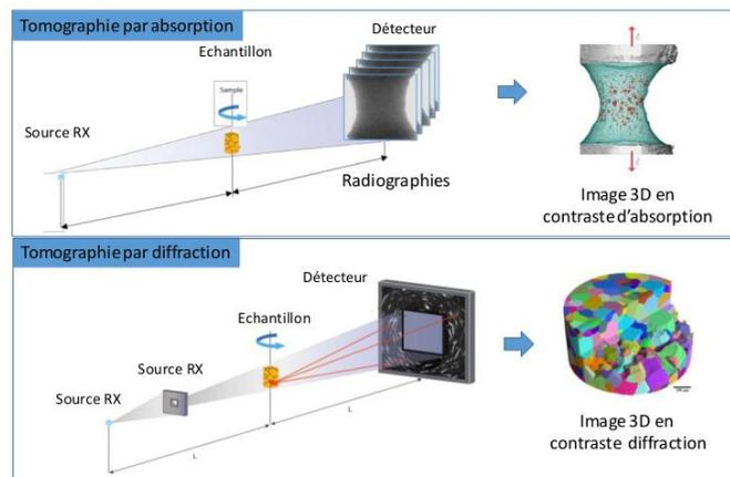
Fig 1 : expected results (a) absorption tomography (b) diffraction contrast tomography (McDonald2015)
